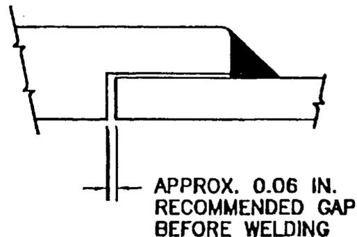
Figure 2 - Welding Gap
